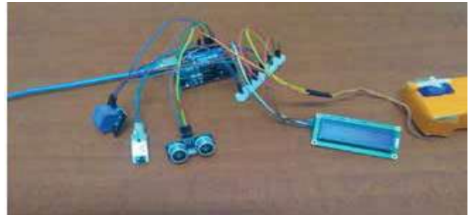
Automatic Hand sanitisation and door control system
